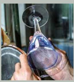
After several hours of cooling in the cooling oven the semi-finished product is ready for cutting. Three types of cut are used on the Splendid set – the stem is cut into edges, a bowl-shaped grinder is used to form a band of bevelled ridges. The most complex is the fine diamond cut, which requires profound concentration, a steady hand and precision work from the cutter.
