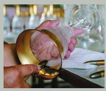
The final treatment follows – after firing, the matt gold plating, both inside and out, polished with agate and haematite to give a more pronounced oroplastique effect.
