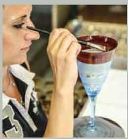
After removing the cover, the band of embossed decoration is painted with a solution of 24-karat gold and fired in a chamber kiln at 560 °C.
