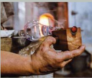
The glassblower forms the glass's stem and base using a special wooden tool.
